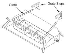
Figure 15 - Installing Grate (Pan Material Not Shown)
